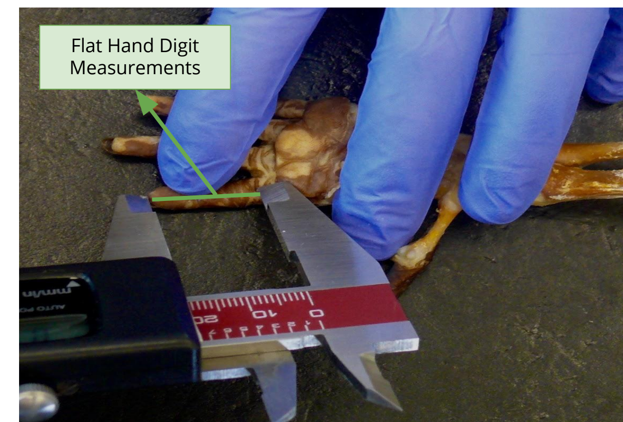
Figure 1. Proximal crease and distal fingertip marking points, used to calculate flat finger length.
